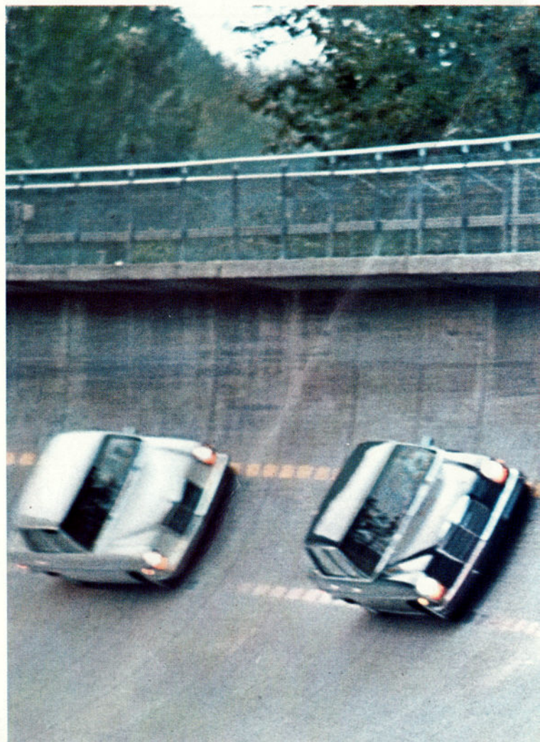
The high wall turn of the Daimler-Benz test track. Where 250s are tested for cornering, braking and high-speed handling.
